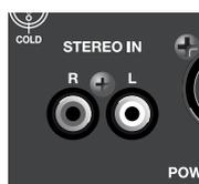
These are RCA phono jacks for inputting analog audio signals from line level equipment. By default they are patched to CH47 and CH48.
