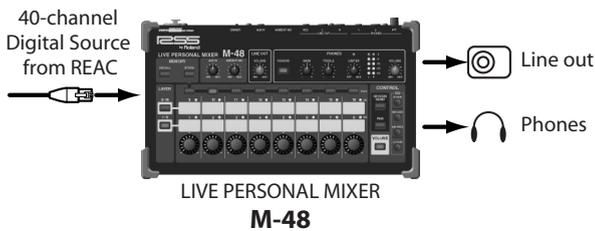
The M-48 provides a REAC port that is able to receive up to 40 channels of digital audio via REAC. The digital audio sources are mixed by the internal 40-channel mixer for monitoring via headphones or monitor speakers.
