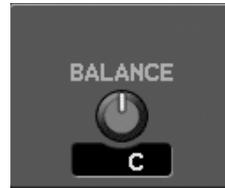
This adjusts the left/right output balance sent from MAIN L/R or stereo-linked AUX/MTX in a range of L63–R63.
