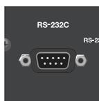
You can use this RS-232C connector to remotely control the M-480 from an external device.
