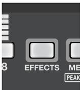
This button accesses the EFFECTS screen where you can control the FX, GEQ, and external inserts. It will light red when the screen is shown.
