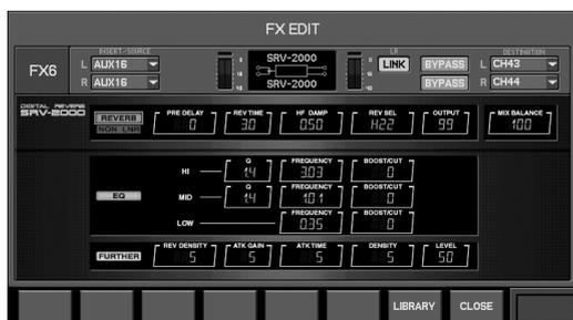
This is a mono-in, stereo-out reverb that models the Roland SRV-2000 MIDI digital reverb. It provides two modes: REVERB mode in which it operates as a conventional reverb, and NON LNR (non-linear) mode in which the reverb sound is cut off according to the gate time setting.
