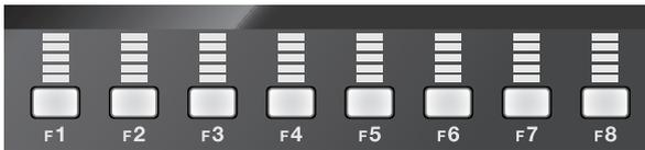
Use these buttons to operate the function buttons shown at the bottom of the display, and to operate the tabs that switch between display screens.
