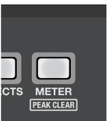
This button accesses the METER screen where you can view the meters. It will light red when the screen is shown.
